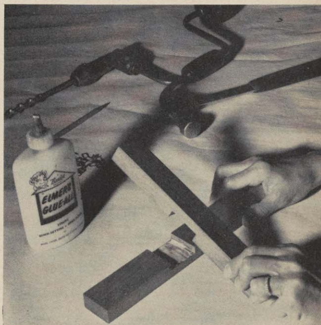
In the second model, a home workshop power saw was pressed into service to make a firmer joint which could be glued together easily to form a neater, stronger holder.
